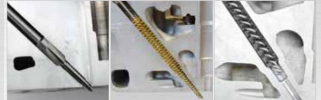
Content: reamers with actuator, adapter guide and 7 brushes (Ø 4.7 mm - 11 mm)
