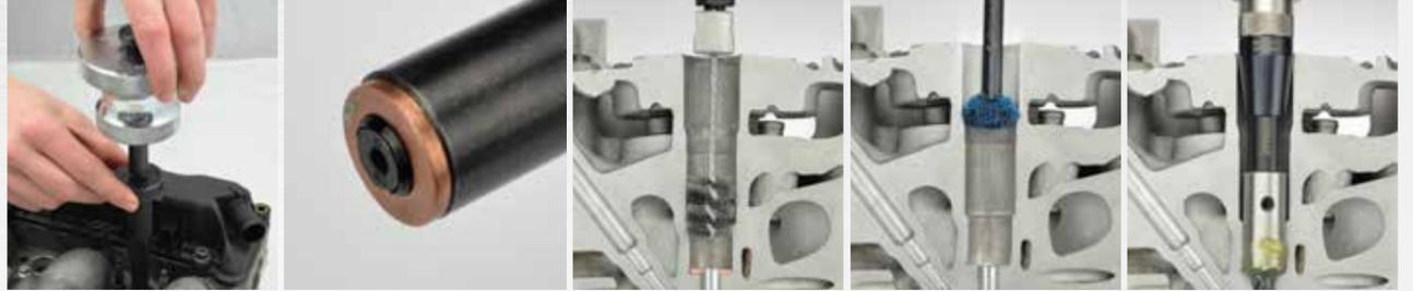
For optimal cleaning and revising the injector shaft. The injector shaft wall, the sealing seat for the injector and the bore for receiving the injector nose are all cleaned with special brushes. In case of severe contamination or damage is the sealing seat precise and controlled revised with the milling tool, in such a way that a perfect sealing surface is reobtained. Seized copper sealing rings can be removed from injector shaft simply and without damage to the cylinder head.
