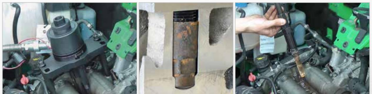
**Use:** For removing frozen common rail injectors from the cylinder head using a 20 ton hollow piston cylinder. If the injector tears during the extraction at the bottom screw connection, it is possible to pull the rest of the injector using the additional extraction spindles.
