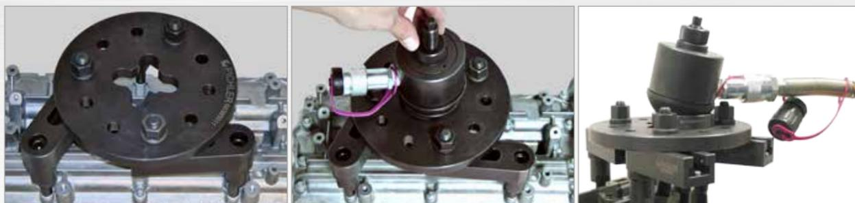
The legs/arms can be adjusted to fit each position in a circle of 300 mm and are individually height adjustable. The adaptors (optionally available) connect the CR-injectors from the various manufacturers (Bosch, Siemens, Delphi, etc.) to the extraction spindle. The injector is extracted from the cylinder head with the tensile force of the 12 ton hydraulic cylinder
