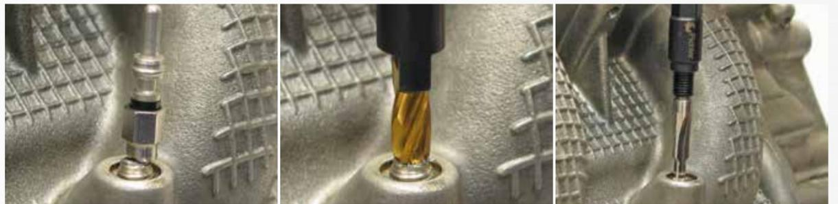
Tools for removing glow plugs and for cleaning or reworking the glow plug hole.
