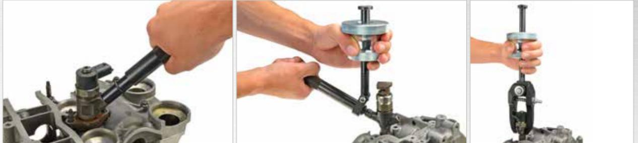
For non-destructive removal of various slightly and moderately jammed injectors.
